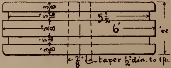
1-#6, Brass Bushing in Cylinder.
